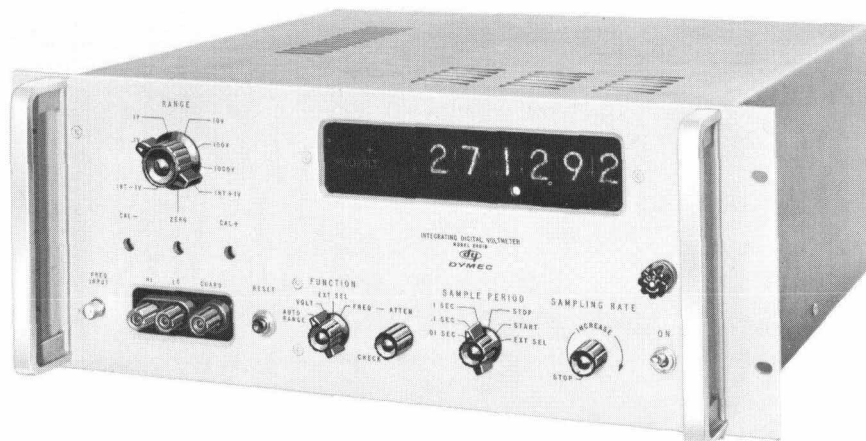
Fig. 3. Dymec Model 2401B Integrating Digital Voltmeter has internal calibration source with stability of \pm 0.01\% per six month period to match voltmeter's high accuracy. Programmable voltmeter has five ranges, from \pm 0.1 to \pm 1000\text{v} full scale, with 300% overranging on four most sensitive ranges for increased resolution and sensitivity on 1-to-3 readings. Guarded, floating input provides high common mode noise rejection; integrating operation averages out superimposed noise and completely eliminates effect of power line hum to retain high accuracy in presence of noise. Overall instrument common-mode rejection is 140 db (10 million to 1) at all frequencies, including dc.
